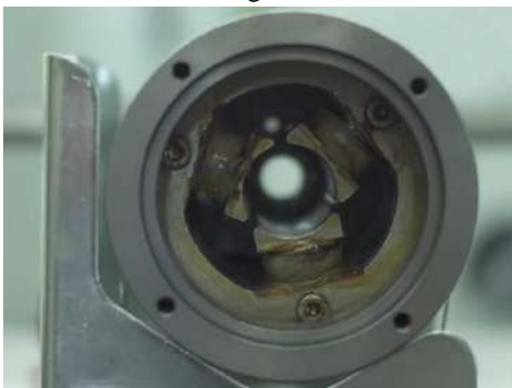
Figure 2. Carbon Nano tubes yarn replacing copper windings [3]
