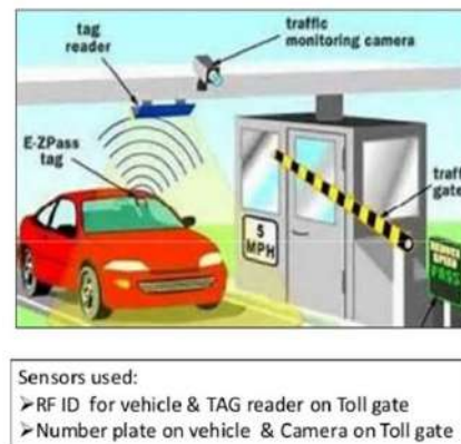
Fig 1. Example of automatic toll collection [6]
