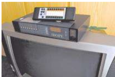
Fig. 2 People-meter with its Remote Control [2]
