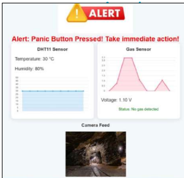
Fig. 4.3. Output when Panic Button is pressed
