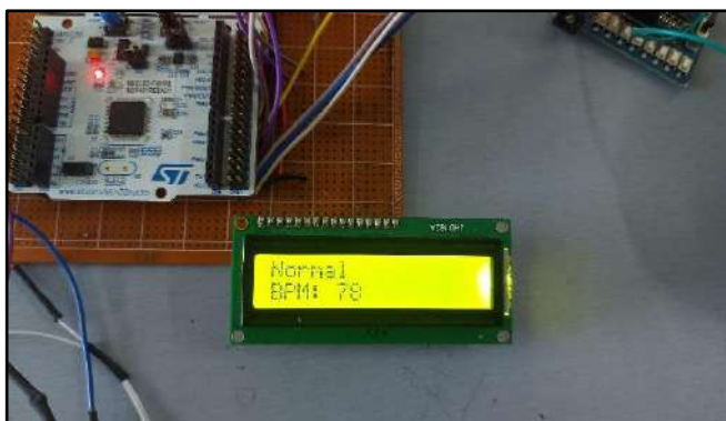
Fig 2.14. Flex and BPM output (no finger is bent)
