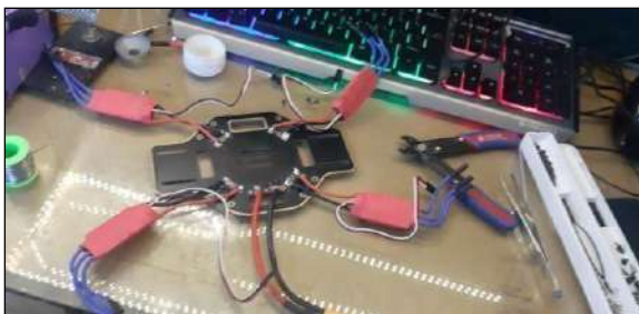
Figure. 8: Basic Connection of Components
