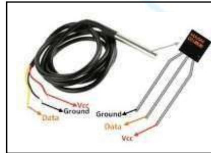
Fig. 7: Temperature Sensor probe (DS18B20)
