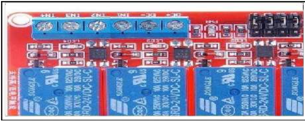
Fig.2: Optocoupler Relay Module
